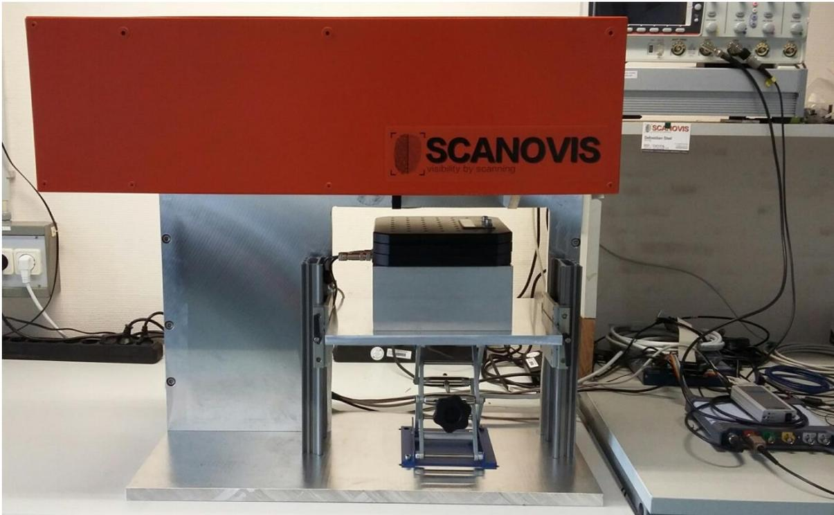
IR Laser Fingerprint Scanner, Prototype
